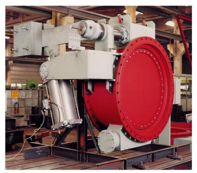
The pictures show the toggle disc valves during tests and trial operations at the Rauenstein works.
