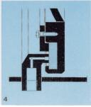
Picture above: Double landing bar with valve disc and sealing element.
